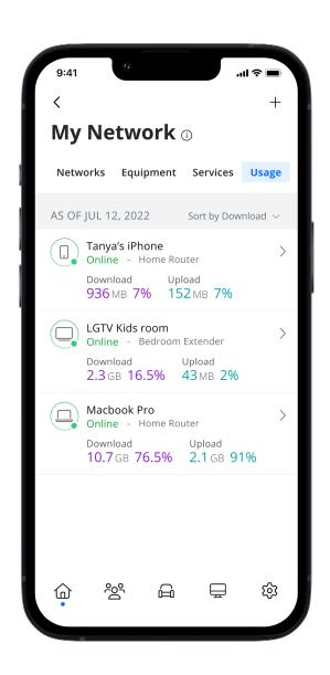
Network Usage is organized by device. From this view, you can see basic information about usage from each Wi-Fi connected device on your network, including: 1. Device identification and whether the device is connected to Wi-Fi 2. What network device it is connected to 3. Network usage 4. The amount of data that has been used by this device Network usage is updated each time you run a bandwidth test through the app.
