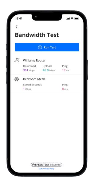
The easiest way to run a bandwidth test is by tapping into "My Network" and then "Bandwidth Test" icon. Then simply tap the Run Test button. The speed test will first run between the GigaSpire and the Internet and then will conduct a speed test between any mesh units and the GigaSpire. Results will show as a notification and update at this location.
